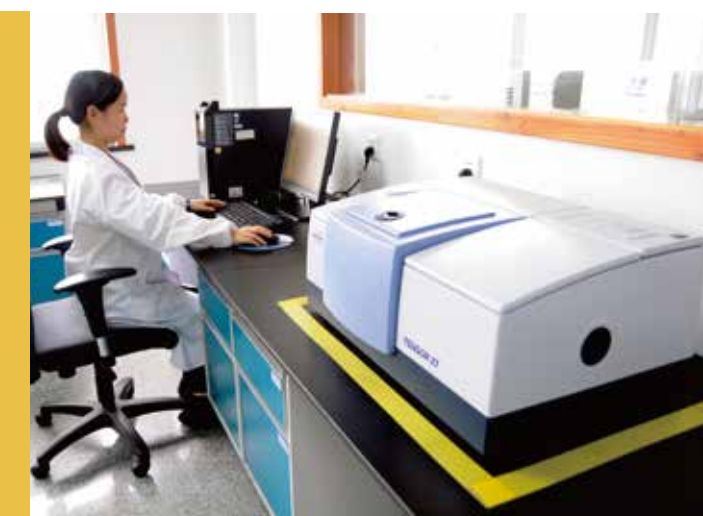
FOURIER TRANSFORM INFRARED SPECTROMETER,FTIR
